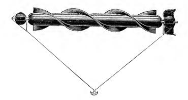
round in a similar manner to convicts in a treadmill. This rotates the whole aërostat, which makes the same advance in the air.
